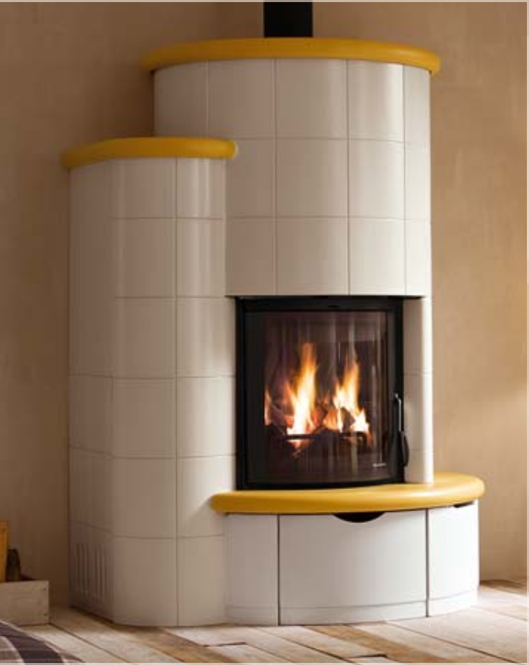
LAURA AIR (also available in the Hydro version). Dimensions: cm 137x90x184h - Weight: kg 450 Global thermal power (performance): kcal/h 14.300 - kW 14 (wood) - kcal/h 12.900 - kW 15 (pellet) Performance: ~77% (wood) ~84% (pellet) Advised quantity of fuel: from 2.5 to 4.5 kg/h (wood) - max 3.7/min 1.2 Kg/h
