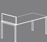
**schermo laterale parziale H 32 (non attrezzabile)** - partial side screen H32 (cannot be used as storage panel) - ecran latéral partiel H32 (non aménageable) - seitliche Teilabschirmung H32 (nicht bestückbar) - panel lateral parcial H32 (no equipable) - painel lateral parcial H32 (não equipável)
